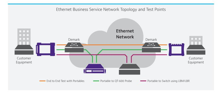
In the diagram above, the "local" T-BERD/MTS is represented on the left side and the "remote" T-BERD/MTS is on the right side. The most common service activation use case is a loop-back of the remote device. In this case, the remote device will be the handheld T-BERD/MTS device.
